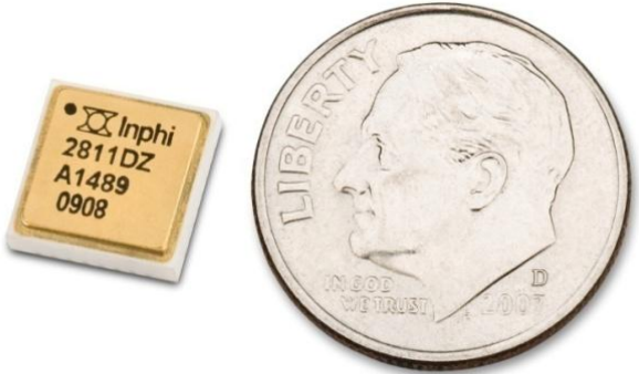
World First Single Chip 40G/100G MZ driver in 7X7 mm 2 SMT package
