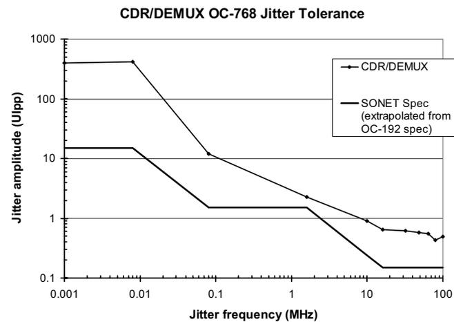
Figure 13.6.5: Measured jitter tolerance.
