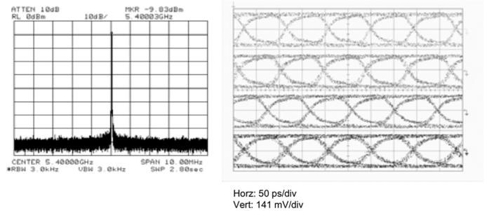
Figure 13.6.4: Recovered clock and demultiplexed data outputs.
