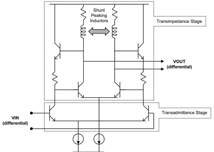
Figure 13.6.2: Limiting amp broadband gain stage schematic.
