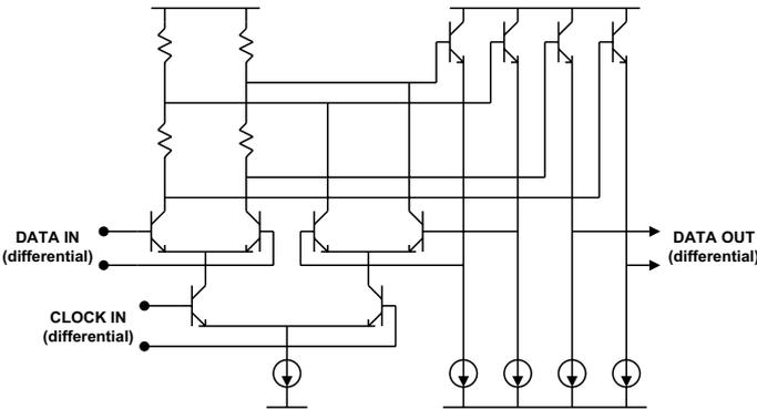
Figure 13.6.3: Split load resistor latch schematic.
