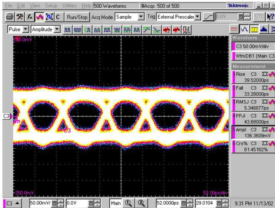
**Figure 3: Electrical eye after 80km of TWRS (inverted TIA output)**
