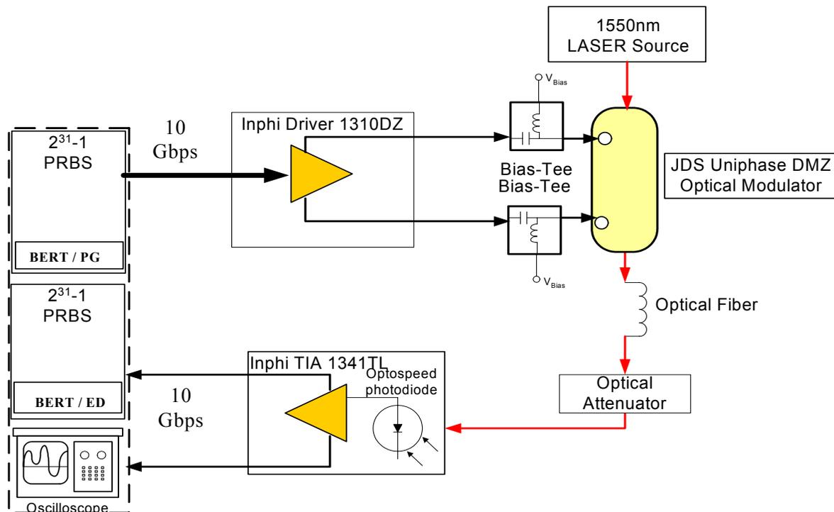
Figure 1: Measurement setup to test Dispersion Penalty
