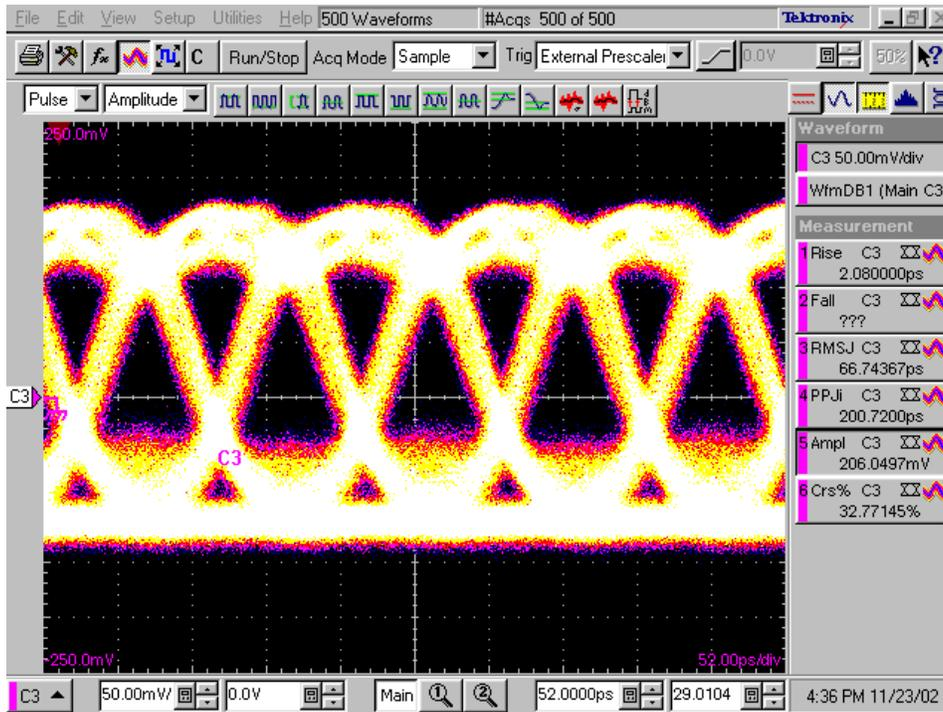
**Figure 2: Electrical eye after 80km of SSMF**
