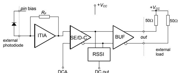
Fig. 9. Block diagram of the TIA chip. *ITIA* – input transimpedance stage, *SE/D-C* – single ended to differential signal converter, *RSSI* – received signal strength indicator, *BUF* – output buffer amplifier, *DCA* – output DC balance adjustment
