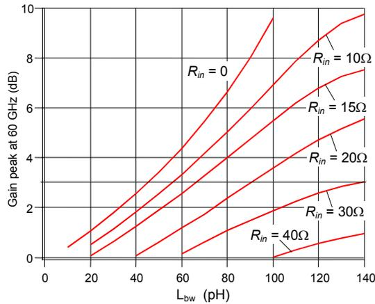
Fig. 4. Gain peaking at  $f = 60$  GHz vs.  $L_{bw}$  for various input resistances  $R_{in}$
