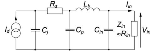
Fig. 3. Model of the TIA input circuit including the photodiode.  $C_j$  – diode junction capacitance,  $R_s$  – diode series resistance,  $C_p$  – contact pad capacitance,  $L_b$  – bonding wire inductance,  $C_{in}$  – input TIA chip capacitance – mostly bonding pad,  $Z_{in}$  – input stage input impedance
