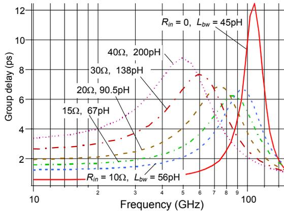
Fig. 5. Group delay vs. frequency for bonding wire inductance selected for 3 dB gain peaking at 60 GHz
