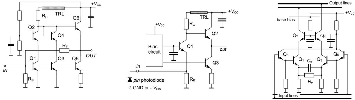
a) input stage for positive input current      b) input stage for negative input current      c) elementary cell of the output buffer
