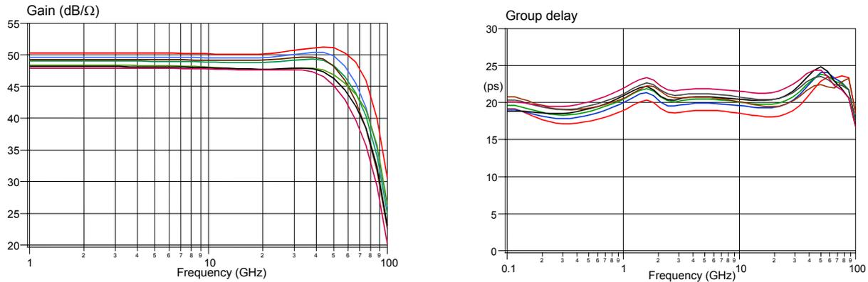
Fig. 6. Simulated gain and group delay for  $-10^{\circ}\text{C} \div +100^{\circ}\text{C}$  operating temperature range and supply voltage changes in the  $3.1\text{V} \div 3.5\text{V}$  range. 600 mV output amplitude version
