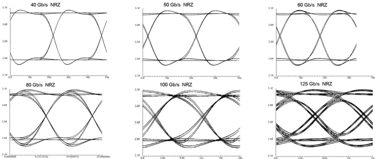
Fig. 7. Simulated eye diagrams for various bit rates (NRZ format) at an input current amplitude of 1 mA
